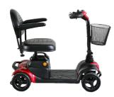
Electrical Scooter Scooter is a 4 wheeled electrical mobility scooter with a top speed of 8 km/h. With a width of 44.5cm, it is easy to maneuver through tight corridors and even within your home.
