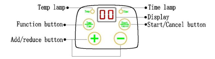
1- Plug the cable in the wall socket, the number "88" will appears as follow, with "di" sounds. And indicates the power is on, and the maker is ready.
