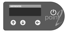
If the enter key ( is pressed for a prolonged time, you enter the programming mode and the menu appears on the display.
